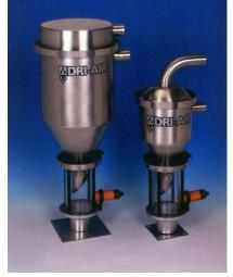
At the start of the loading sequence, the proximity switch on the receiver senses there is no material. The blower starts, and the loader valve on the inlet line to the blower is opened. Because the receiver is sealed, a vacuum is created within the takeoff box, pulling material from the hopper.
